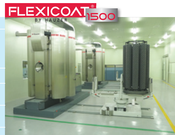
Flexicoat® 1500, mass production equipment for component makers and job coaters
